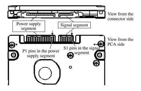
Figure 3.8 Power supply pins (CN1)
